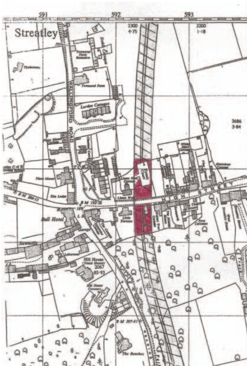
Section of the Streatley by-pass plan showing the tunnel (in red) under the High Street [Mike Brodie]
